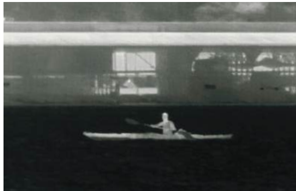
Thermal imaging instantly detects kayaks, paddleboards, and personal watercraft. The kayaker's own body heat makes him a bright target for FLIR thermal imaging.
